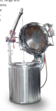
500 lb stainless steel wet digester with an automatic locking ring lid and removable basket for ease of operation.
