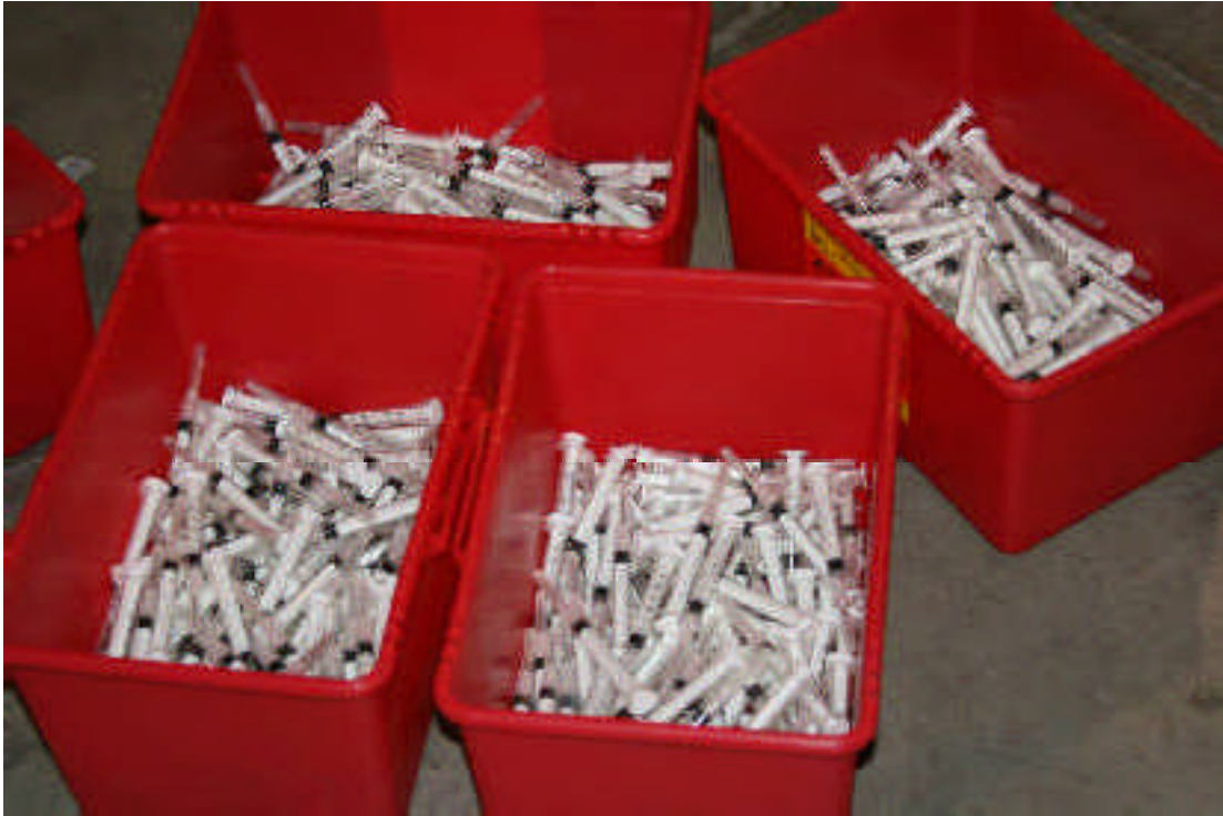
Figure #5 – Small (3.5 gal) sharps containers loaded with biological indicators and unused sharps – to allow for view, tops were removed.
