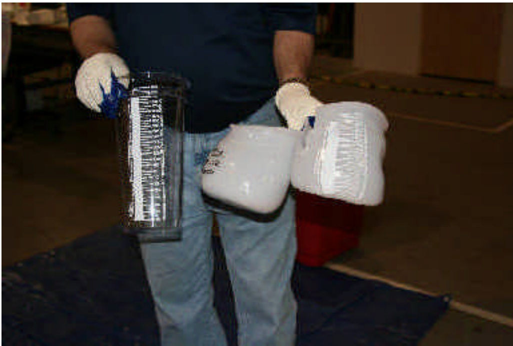
Figure #12 – Autoclavable suction canister on left and non-autoclavable one on right after treatment in the VariClave
