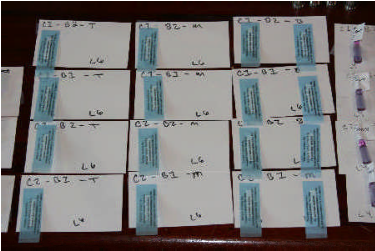
Figure #3. An enlarged view of the 10^4 and 10^6 spore strips used in the efficacy tests of the VariClave.
