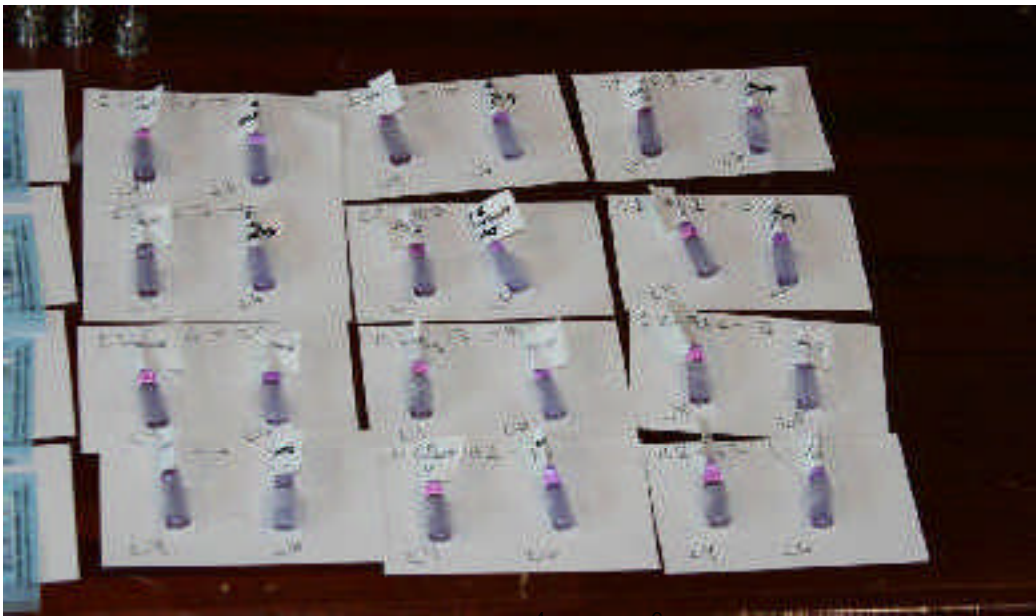
Figure 2. An enlarged view of the 10 -4 and 10 -6 spore ampoules employed in the efficacy studies of the VariClave.
