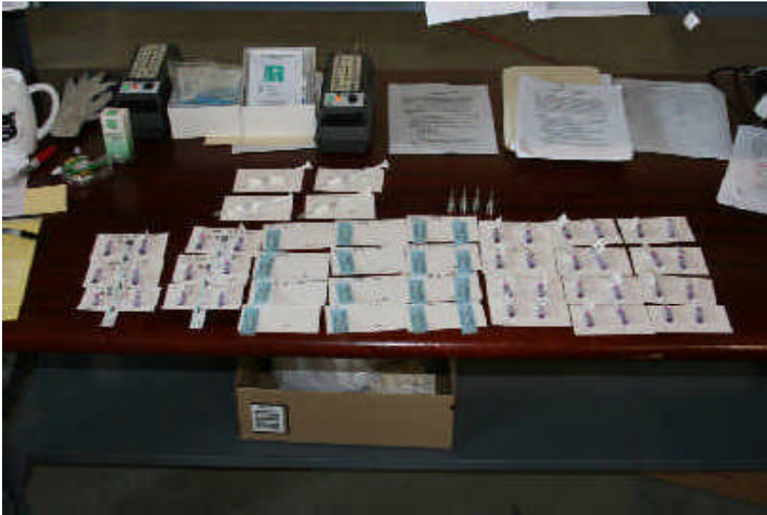
Figure #1. View of the different types of biological indicators, i.e., spore ampoules, spore strips, syringes load with spore suspensions, employed in the efficacy studies of the VariClave.
