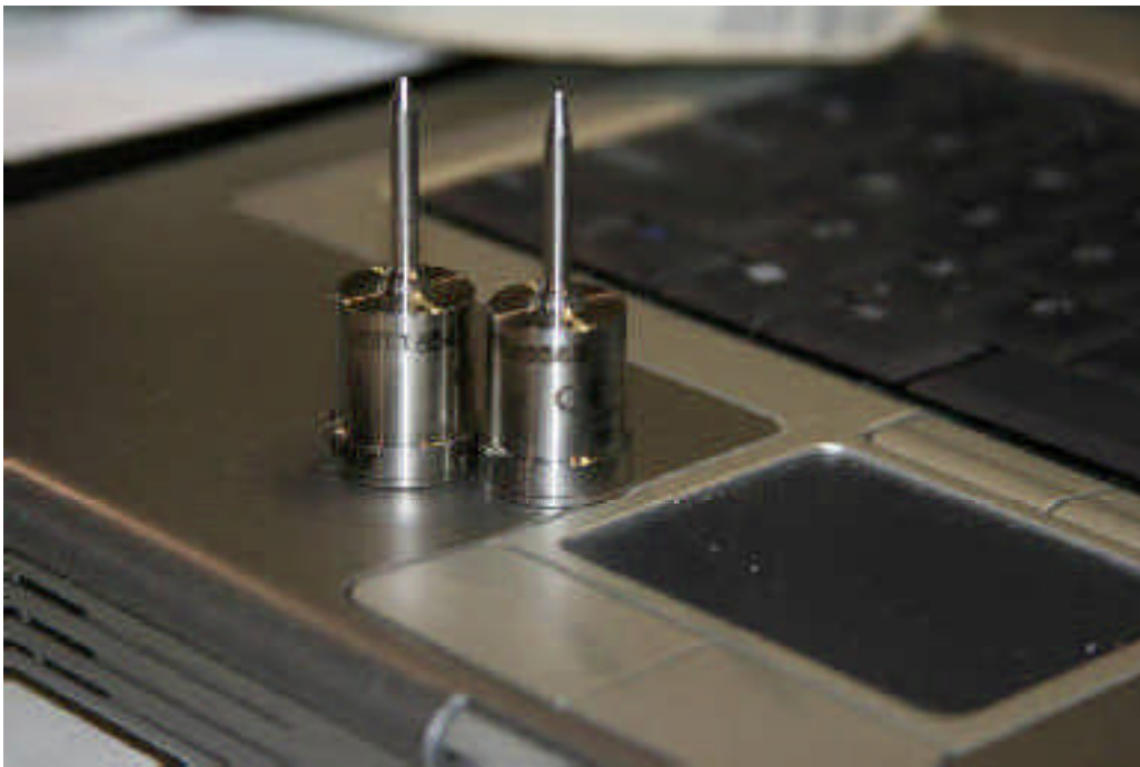
Figure #8 – Data tracers as used to gather temperature data within the autoclave and within the test containers
