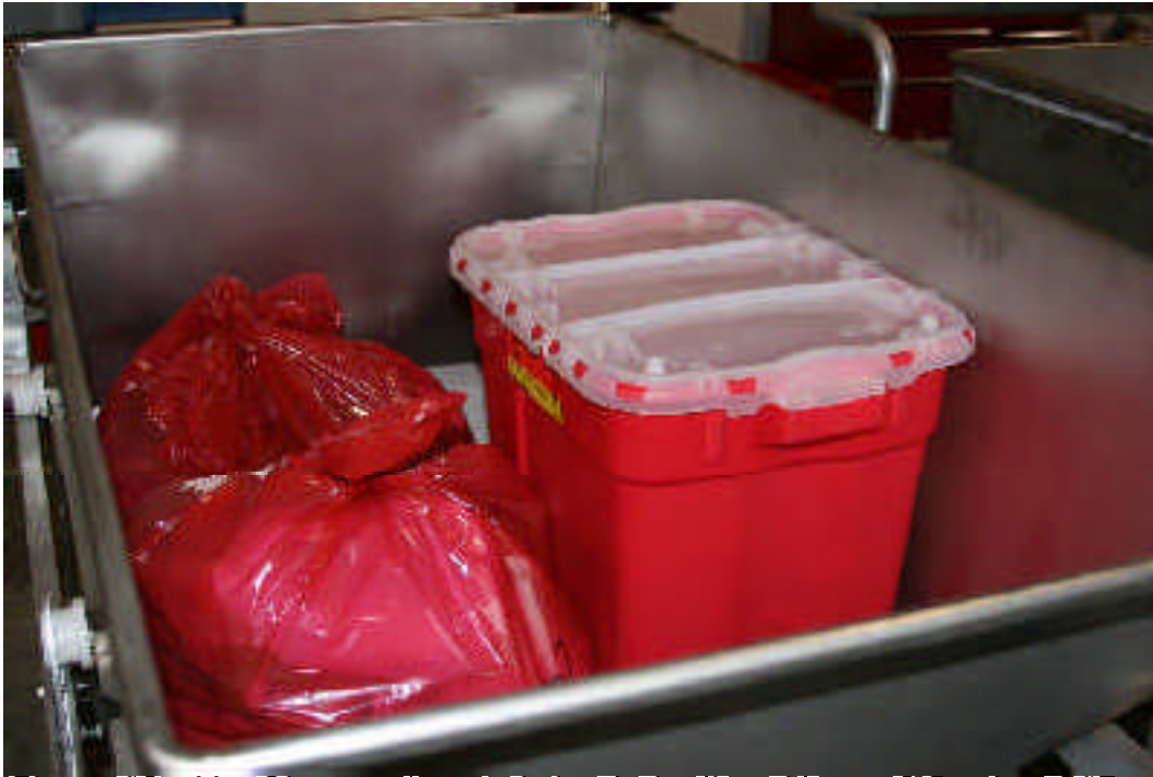
Figure #9 – Var Clave cart partially loaded with red bags, 3.5 gal and 17 gal sharps containers.
