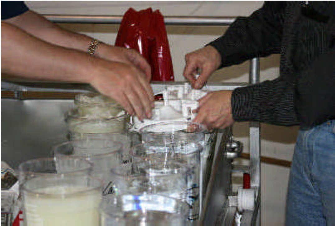
Figure #7 – Preparation of suction cartridges with different solidifying agents
