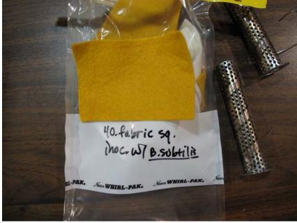
of the STI unit, along with the bulk wood chips. Treated samples were collected from the waste, placed in labelled plastic bags and frozen within 15 minutes after the samples were collected from the waste.
