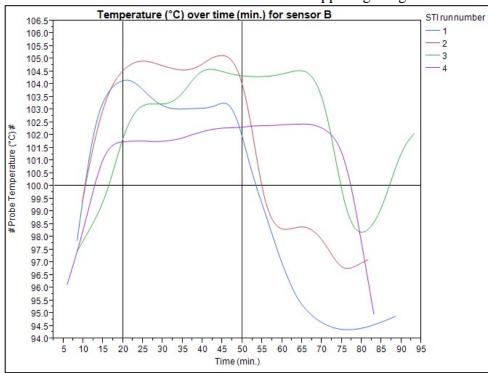
The black horizontal reference lines in the graphs show the 212 F (100 C) threshold. All the colored lines are above 212 F (100 C), when referenced to the two vertical reference lines. The two vertical reference lines in the graphs represent the 30 minutes required by the USDA
