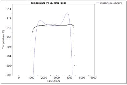
temperature of the hay at 15 sec intervals over a 1.5 hour time period. The average temperature of the hay inside the auger was 210.5 F (99 C), for approximately 50 minutes
