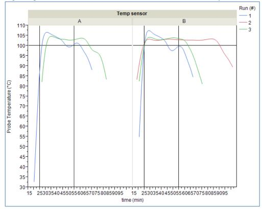
The two sensors were labeled A and B on the top x-axis, and the three test runs are labelled by three colored lines in the upper right legend. Temperature (C) is on the y-axis, and time (min.) is on the bottom x-axis. The average temperatures and exposure time, when the waste temperature was above 212 F (100 C), was estimated from the data (Table 5).
