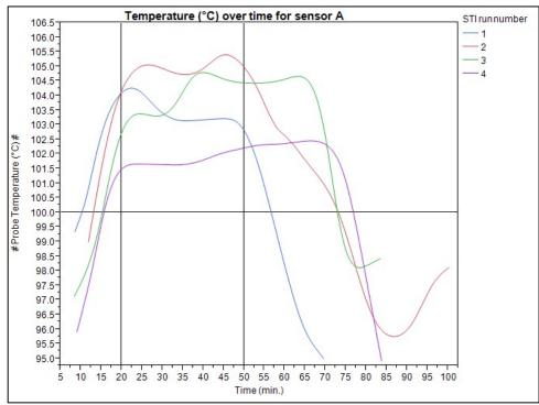
Figure 6. Average temperature (C), graphed over time, for each of the four STI runs for sensor A. The color coded label for the four tests is in the upper right legend.
