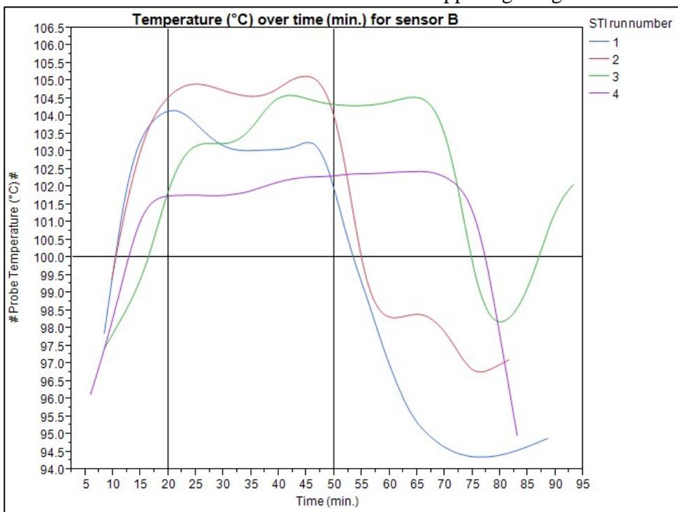
The black horizontal reference lines in the graphs show the 212 F (100 C) threshold. All the colored lines are above 212 F (100 C), when referenced to the two vertical reference lines. The two vertical reference lines in the graphs represent the 30 minutes required by the USDA
