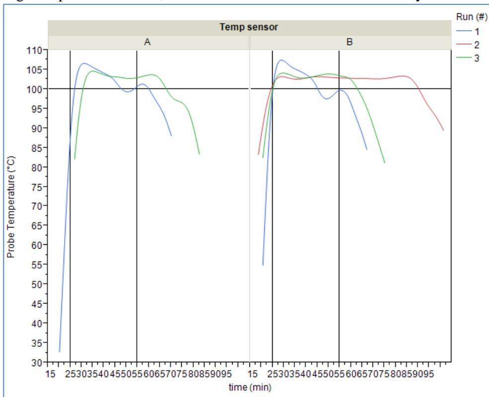
The two sensors were labeled A and B on the top x-axis, and the three test runs are labelled by three colored lines in the upper right legend. Temperature (C) is on the y-axis, and time (min.) is on the bottom x-axis. The average temperatures and exposure time, when the waste temperature was above 212 F (100 C), was estimated from the data (Table 5).
